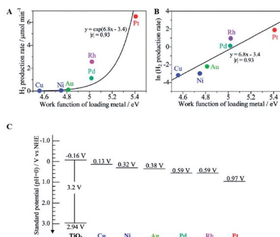
Fig. 3 Relationship between the hydrogen production rate over the  $\text{M}(0.1)/\text{TiO}_2$  samples and the work function of the corresponding bulk metal (A), the logarithmic plot (B), and the standard potentials for the band edge positions of titanium oxide and the Fermi level of each loading metal (C). Reprinted with permission from ref. 62. Copyright 2012 American Chemical Society.
