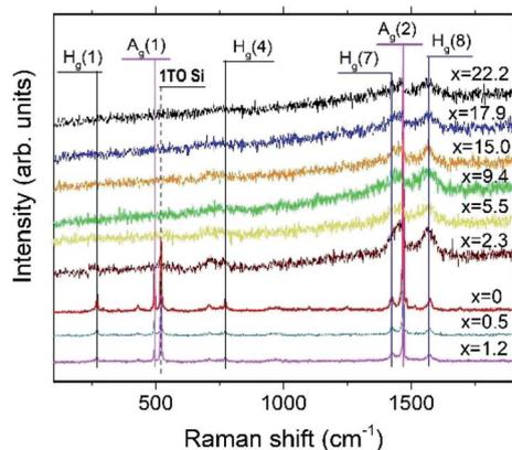
Fig. 9 Raman spectra of the  $\text{Au}_x\text{C}_{60}$  films with different Au concentrations ( $x$ ). The  $x$  values are shown for the respective spectra. Some of the  $\text{C}_{60}$  vibration modes with  $A_g$  and  $H_g$  symmetry are indicated by vertical lines. The position of the intense 1TO Si(100) mode is indicated by the dashed vertical line (see text).
