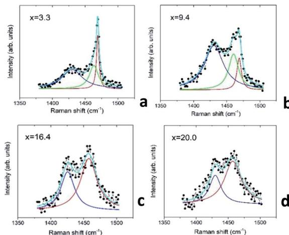
Fig. 10 Raman spectra of the  $\text{Au}_x\text{C}_{60}$  mixture films near the positions of the  $H_g(7)$  and  $A_g(2)$  modes of  $\text{C}_{60}$ : (a and b) the mixture films from the interval R2; (c and d) the mixture films from the interval R3. The experimental spectra (black dots) fitted by a superposition of Lorentzians (light-blue line). See description in the text.
