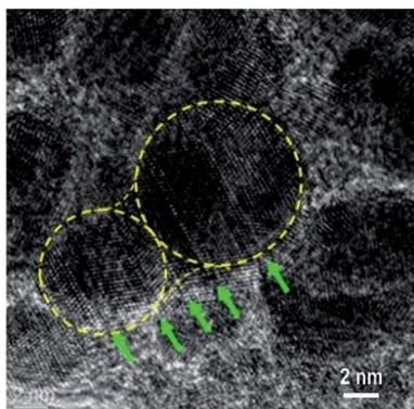
Fig. 5 HRTEM image of nanostructures at the edge of the sample S8 ( $x = 16.4$ ). The Au NP with irregular shape seen in the centre of the image is a coalescence of two NPs with different sizes. The crystal twinning in the Au NPs is seen. The position of the {111} twin boundaries in the Au NPs is indicated by green arrows. The crystal lattice in the Au NPs is well observed as the (111) plane in the twinned crystals.
