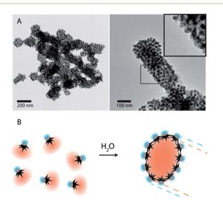
Fig. 3 (A) TEM images of nanoparticle-amphiphile assemblies (Fig. 1B1) with long thiol-terminated PS ( $M_W$ : 20 kg mol<sup>-1</sup>). Inset shows the Janus nanoparticles with the Fe<sub>3</sub>O<sub>4</sub> facing the exterior of the assemblies. (B) Schematic representation of a self-assembly process by solvent exchange and the formation of assemblies where the Au nanostars are facing the hydrophobic core and the hydrophilic Fe<sub>3</sub>O<sub>4</sub> is facing the exterior.
