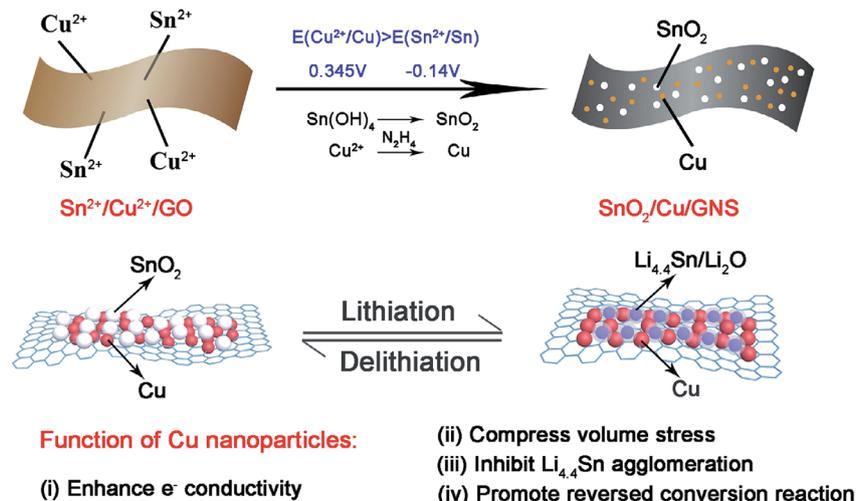
Fig. 2 Schematic illustration of the selective reduction fabrication of SnO<sub>2</sub>/Cu/GNS composite; structure evolution and functions of Cu nanoparticles during lithiation and delithiation processes. Reproduced with permission from Jiang *et al.*, 2019. Copyright 2019, Elsevier.
