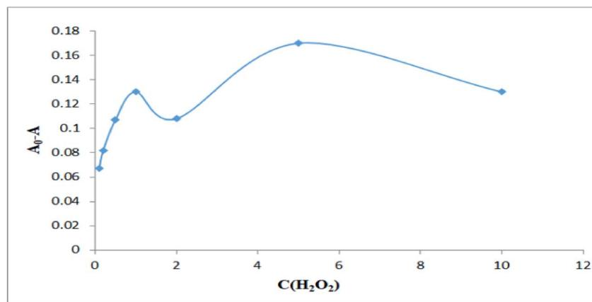
Fig. 3 Effect of H<sub>2</sub>O<sub>2</sub> on the generation of hydroxyl radicals from samples containing 3 mL of  $1.5 \times 10^{-4}$  mmol 4,  $3.375 \times 10^{-5}$  mmol methylene blue and H<sub>2</sub>O<sub>2</sub> at different concentrations. Reproduced with permission from Li *et al.*, 2019. Copyright 2019, Royal Society of Chemistry.
