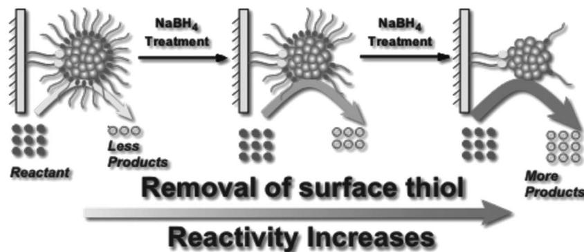
Fig. 7 Illustration of enhanced catalytic activity in a selective oxidation reaction with supported thiolate-stabilized  $\text{Au}_{25}(\text{SR})_{18}$  cluster catalysts by mild chemical stripping of their surface ligands with  $\text{NaBH}_4$ . Reprinted with permission from ref. 82. Copyright 2014 John Wiley and Sons.
