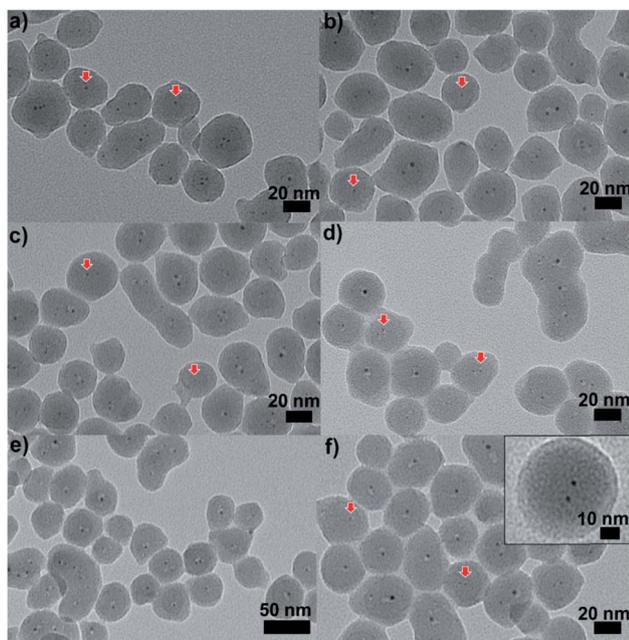
Fig. 9 TEM images of Au<sub>25</sub>@SiO<sub>2</sub> materials calcined at (a) 250 °C, (b) 350 °C, (c) 450 °C, (d) 550 °C, and (e) and (f) 650 °C (inset: enlarged image). Reproduced with permission of the Royal Society of Chemistry.<sup>100</sup>
