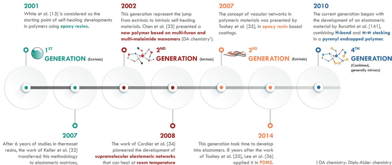
Fig. 3 Timeline of generations in self-healing polymers.
