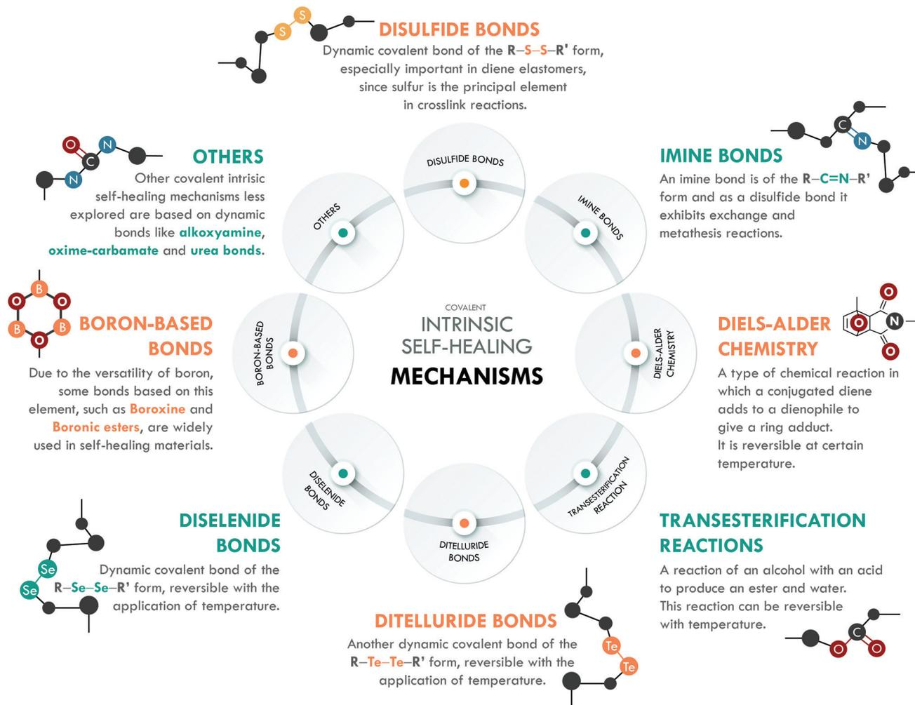
Fig. 8 Covalent intrinsic self-healing mechanisms.
