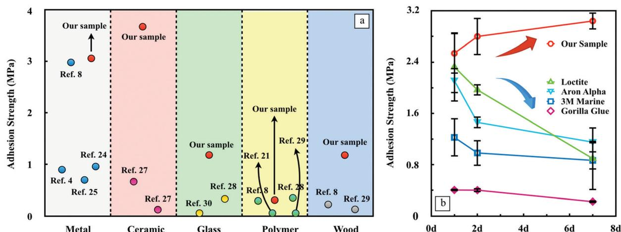
Fig. 4 Benchmarking underwater bonding performance of nanocomposite adhesives. (a) Underwater bonding of nanocomposite adhesives compared to other adhesives reported in the literature. (b) Adhesion strength of nanocomposite adhesives as a function of time used underwater in comparison with the commercial products. Lap shear joints were between aluminum substrates.
