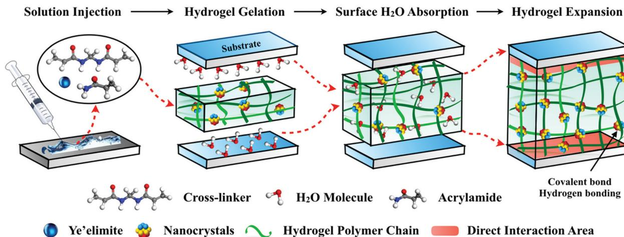
**Fig. 1** Design of nanocrystal reinforced hydrogel networks. The monomer, crosslinker, and ye'elimite were simply blended to fabricate a nanocomposite PAM hydrogel solution, which was directly injected under water to the substrates. During gelation, the water molecules at the interfaces were captured into the hydrogel matrix, forming a sound bonding between the adhesives and the substrates.
