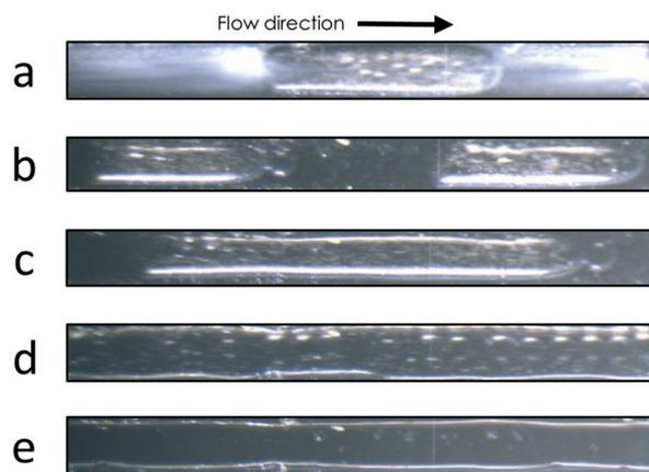
Fig. 4 Temperature-induced tuning of different flow patterns. Observed flow patterns at a fixed flow rate (70  $\mu\text{l min}^{-1}$ ) and channel cross section (700  $\times$  700  $\mu\text{m}^2$ ) with temperature as the only experimental variable: a) -1 °C, b) 5 °C, c) 10 °C, d) 15 °C and e) 20 °C. black arrow indicates flow direction.
