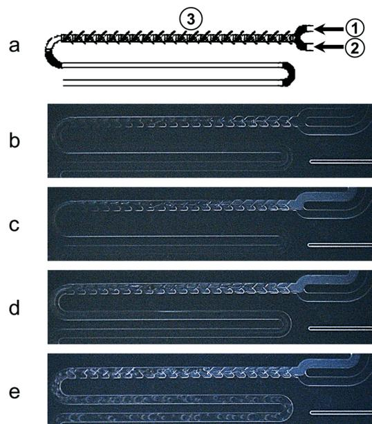
**Fig. 1** Temperature-dependent mixing of 5CB and MeOH, infused at the top (a1) and bottom (a2) inlet, respectively. Passive mixing is induced *via* a static micromixer with staggered oriented ridges (a3). (b–e) Snapshots of the microfluidic chip at various temperatures: 40 °C (b); 35 °C (c); 24 °C (d) and 12 °C (e).
