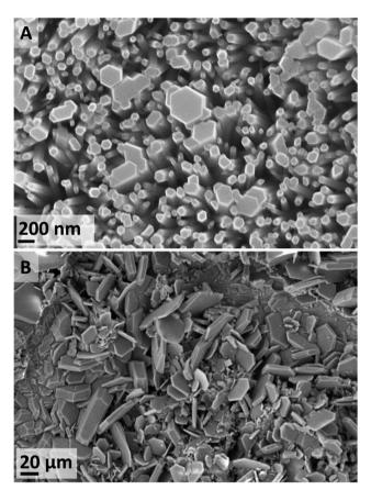
Fig. 4 Magnified zinc surface exposed to [C<sub>4</sub>C<sub>1</sub>im]Cl (IL-1,  $X_{\rm H_2O}=0.98$  solution at 70  $\pm$  1 °C). (A) ZnO nanorods after 4 d exposure (magnification 134.17k×) (average size 90  $\pm$  40 nm, n=361). (B) ZHC plate-like crystals after 15 d exposure (magnification 1.44k×). Estimated thickness 2.5  $\pm$  1.5  $\mu$ m (n=85), diameter 19  $\pm$  8  $\mu$ m (n=85).
