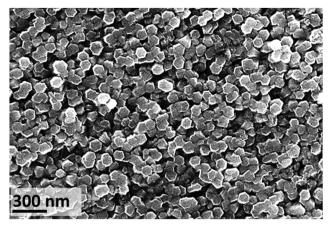
Fig. 7 SEM image of zinc substrate after exposure to [C<sub>4</sub>C<sub>1</sub>im]Cl (IL-1,  $X_{\rm H_2O}$  = 0.75 solution, 20  $\pm$  1 °C) for 26 d, showing the top of hexagonal nanorods (average size 150  $\pm$  30 nm, n = 278).
