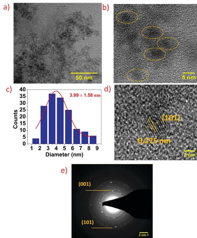
Fig. 2 (a and b) TEM image of the synthesized SnS<sub>2</sub> QDs, (c) size distribution of SnS<sub>2</sub> QDs, calculated average diameter of SnS<sub>2</sub> QDs is 3.99 ± 1.58 nm, (d) HRTEM lattice fringes of SnS<sub>2</sub> QDs, and (e) SAED pattern of SnS<sub>2</sub> QDs.
