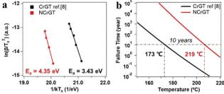
Fig. 7 (a) Kissinger plots for the activation energy calculation of the CrGT and NCrGT films and (b) temperature-dependence of failure time te 10% for the GCT and GST films
