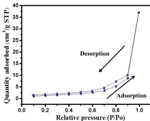
Fig. 5  $\text{N}_2$  adsorption-desorption curve of  $\text{CaTiO}_3$  pyramids.
