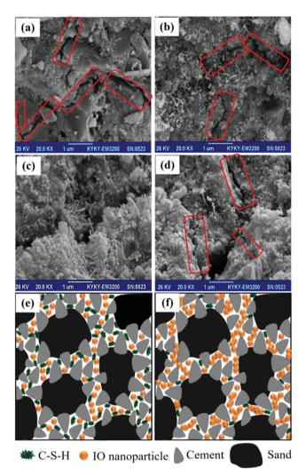
**Fig. 3** High-magnification SEM images of cement mortars with different iron oxide contents: (a) 0.0 wt%, (b) 2.0 wt%, (c) 2.5 wt% and (d) 3.0 wt%. Schematic visualization of (e) uniformly dispersed iron oxide nanoparticles and (f) agglomerated iron oxide nanoparticles in the cement mortar matrix.
