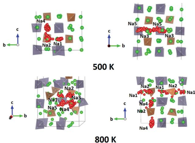
Fig. 7 Typical  $\text{Na}^+$  ion trajectories in  $\text{Na}_{11}\text{Sn}_2\text{PS}_{12}$  at  $T = 500$  K (top row) and  $800$  K (bottom row). Diffusion occurs in all three dimensions. Grey (brown) tetrahedra represent  $\text{SnS}_4$  ( $\text{PS}_4$ ). Spheres represent Na sites, among which those marked in red correspond to Na sites along the selected trajectories.
