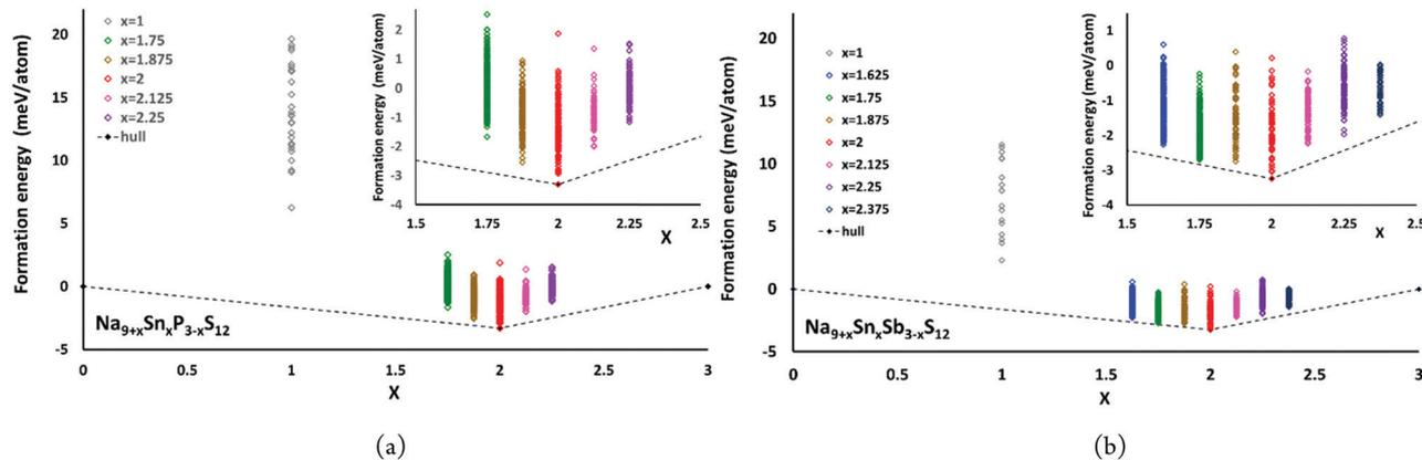
Fig. 5 The convex hulls for (a)  $\text{Na}_{9+x}\text{Sn}_x\text{P}_{3-x}\text{S}_{12}$  at  $x = 0$ ,  $x = 1$ ,  $1.75 \leq x \leq 2.25$  and  $x = 3$  as well as (b)  $\text{Na}_{9+x}\text{Sn}_x\text{Sb}_{3-x}\text{S}_{12}$  at  $x = 0$ ,  $x = 1$ ,  $1.625 \leq x \leq 2.375$  and  $x = 3$ .
