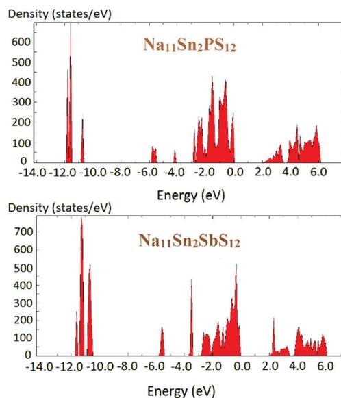
Fig. 6 Density of states of  $\text{Na}_{11}\text{Sn}_2\text{PS}_{12}$  and  $\text{Na}_{11}\text{Sn}_2\text{SbS}_{12}$ .
