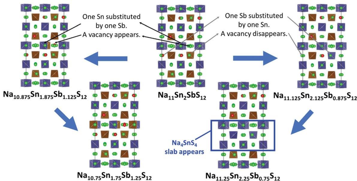
Fig. 4 Schematic representation of derivation of the  $\text{Na}_{9+x}\text{Sn}_x\text{Sb}_{3-x}\text{S}_{12}$  structures with  $x = 1.75, 1.875, 2.125$  and  $x = 2.25$ . Blue (brown) tetrahedra represent  $\text{SnS}_4$  ( $\text{SbS}_4$ ), green spheres occupied Na sites. Na vacancies are marked in red. For  $\text{Na}_{11.25}\text{Sn}_{2.25}\text{Sb}_{0.75}\text{S}_{12}$  the lowest energy structure contains a slab of  $\text{Na}_4\text{Sn}_4$  composition marked in blue.
