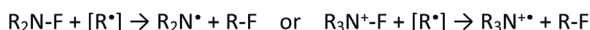
Scheme 5 SET process between alkyl radical species and fluorinating agent yielding an R–F species.
