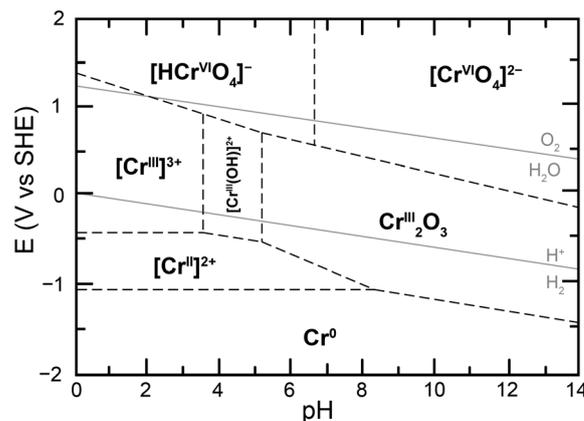
Fig. 2 Proposed calculated Pourbaix diagram for chromium at  $10^{-6}$  M total dissolved chromium and 25  $^{\circ}\text{C}$ , adapted from ref. 20.
