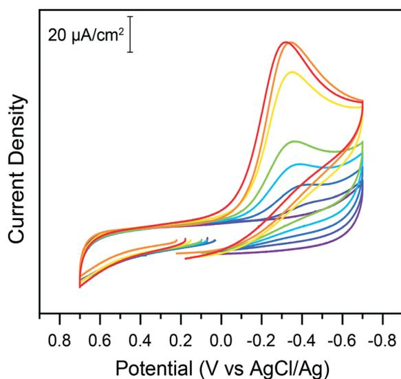
Fig. 1 Cyclic voltammograms on glassy carbon electrodes of a 200  $\mu\text{M}$  solution of potassium chromate in water in the absence (purple) and presence of increasing concentrations of citric acid: 0.05 mM (dark blue), 0.1 mM (light blue), 0.15 mM (cyan), 0.2 mM (green), 0.3 mM (yellow), 0.4 mM (orange), and 0.5 mM (red). Data recorded at 100  $\text{mV s}^{-1}$ .
