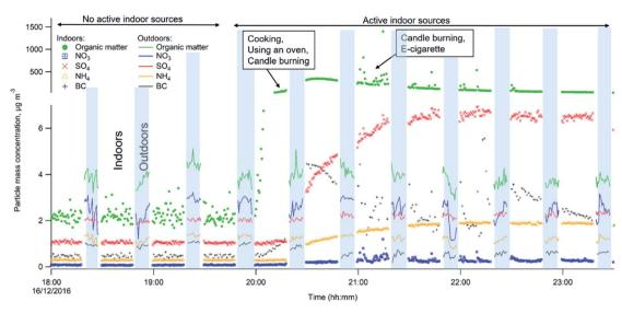
Fig. 3 Particle mass concentrations of different chemical fractions during no active indoor sources (18:00–19:45), and with active indoor sources periods (19:45–24:00) inside and outside the residence during one evening. The changing pattern represents measurements with the switching valve alternating between indoors (starting position in this graph, no shading, 20 min) and outdoors (marked with shading, 10 min). Note the scale change on the Y-axis.
