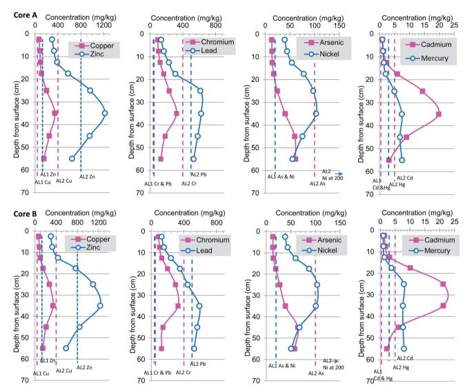
ig. 4 Heavy metal concentrations profiles for cores A and B. Dashed vertical lines represent non-statutory sediment quality guidelines
