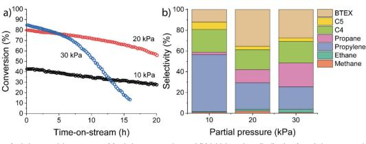
Fig. 5 Influence of ethylene partial pressure on (a) ethylene conversion and (b) initial product distribution for ethylene conversion over HZSM-5 measured after 15 minutes time-on-stream (reaction conditions: T = 500 °C; atmospheric pressure; carrier flow 50 mL min<sup>-1</sup> He).
