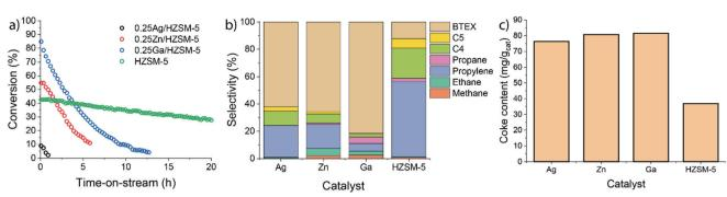
Fig. 2 (a) Conversion of ethylene as a function of time-on-stream; (b) the initial product distribution in the reaction of ethylene on parent and metal-modified 0.25 M/HZSM-5 zeolites measured after 15 min time-on-stream; (c) total coke content in used catalyst samples measured with TGA (reaction conditions: 500 °C, atmospheric pressure; ethylene partial pressure 10 kPa; carrier flow 50 mL min<sup>-1</sup> He, WHSV =  $3.75 \text{ h}^{-1}$ ).
