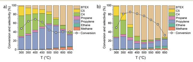
Fig. 4 Influence of temperature on the initial ethylene conversion (measured after 15 min time-on-stream) and the product distribution during ethylene conversion over (a) HZSM-5 and (b) 0.25Ga/HZSM-5 zeolites (reaction conditions: 500 °C; atmospheric pressure; ethylene partial pressure 10 kPa; carrier flow 50 mL min<sup>-1</sup> He, WHSV =  $3.75 \text{ h}^{-1}$ ).
