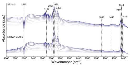
Fig. 7 Evolution of IR spectra in time upon adsorption of ethylene on HZSM-5 and 0.25Ga/HZSM-5 zeolites at 50 °C. The spectra are taken every 2.5 min; ethylene partial pressure 10 kPa.
