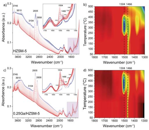
Fig. 8 IR spectra and heat maps of low wavenumber region (1800-1300 cm<sup>-1</sup>) recorded during TPR during exposure to ethylene on (a and b) HZSM-5 and (c and d) 0.25Ga/HZSM-5 zeolites during heating from 50 °C to 500 °C (colour transition from blue to red on the graphs a and c).
