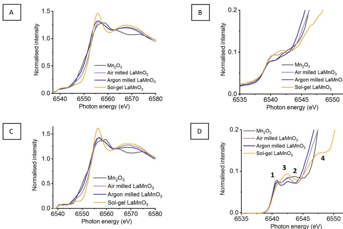
Fig. 7 (A) Mn K-edge XANES with (B) highlighted pre-edge region compared to (C) HERFD-XANES with (D) highlighted pre-edge region of mechanochemical synthesis of  $\text{LaMnO}_3$  within air and argon environments compared to sol-gel  $\text{LaMnO}_3$  and precursor  $\text{Mn}_2\text{O}_3$ .
