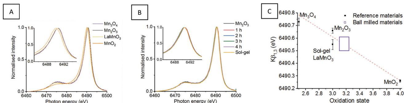
**Fig. 2** Mn Kβ XES mainlines for (A) Mn reference oxides and sol-gel synthesised LaMnO<sub>3</sub> with (B) 'time-slices' during the mechanochemical synthesis of LaMnO<sub>3</sub> (C) presents the Kβ<sub>1,3</sub> max as a function of oxidation state, with a line of best fit calculated from the reference materials and used to calculate the oxidation state of the ball milled materials.<sup>11</sup>
