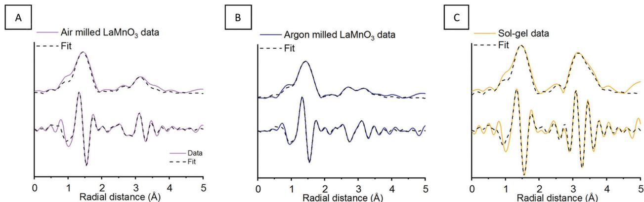
Fig. 6 Mn K-edge EXAFS data after 4 h of milling in (A) atmospheric and inert (B) milling conditions showing the magnitude and imaginary components of the  $k^2$ -weighted FT data and fits compared to (C) sol-gel synthesised  $\text{LaMnO}_3$ .
