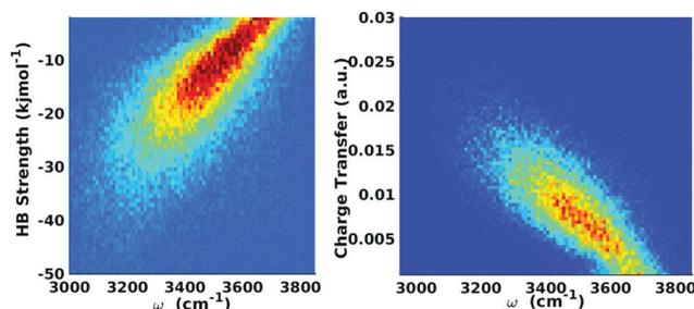
Fig. 9 Equilibrium distributions of OH stretch frequency versus HB strength, as quantified by the  $\Delta E_{CT}$  terms (left) and the associated charge-transfer terms ( $\Delta Q_{CT}$  in units of elementary charge, right). The frequencies of the OH modes were calculated using a wavelet-based time-series analysis.<sup>18,50,51</sup> Reproduced from ref. 18/CC BY.
