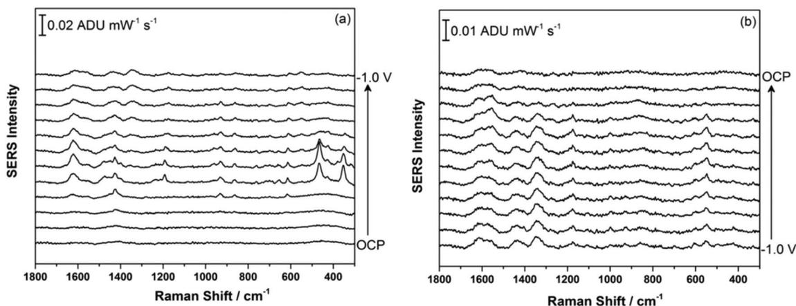
Fig. 2 (a) EC-SERS signal for THC on the AgNP-modified SPE at OCP, and then from 0.0 to  $-1.0$  V in 100 mV increments. (b) EC-SERS signal stepping back from  $-1.0$  V to 0.0 V in 100 mV increments, and finally at OCP measured after the potential stepping. Spectra measured at 780 nm, 80 mW, 30 seconds.
