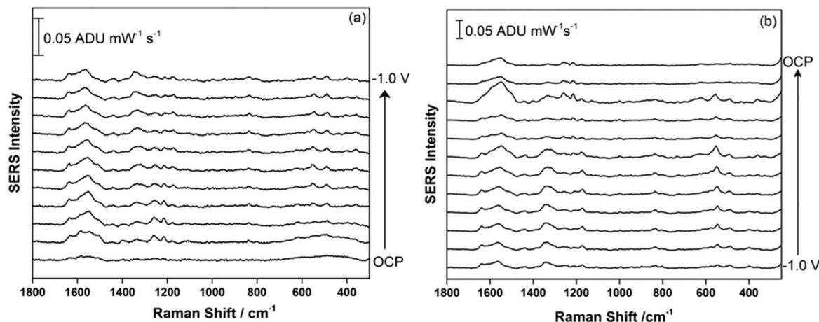
Fig. 4 (a) EC-SERS signal for THC-COOH on the AgNP-modified SPE at OCP, and then from 0.0 to  $-1.0$  V in 100 mV increments. (b) EC-SERS signal stepping back from  $-1.0$  V to 0.0 V in 100 mV increments, and finally at OCP measured after the potential stepping. Spectra measured at 780 nm, 80 mW, 30 seconds.
