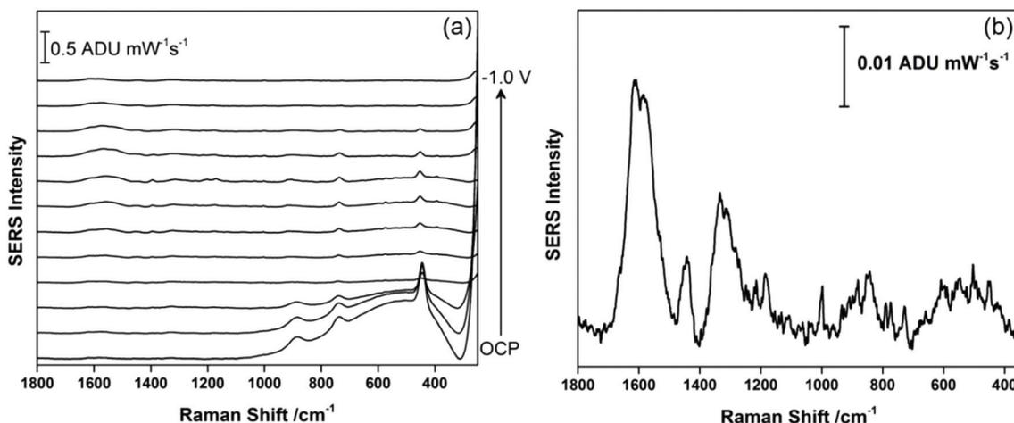
Fig. 6 (a) EC-SERS progression (cathodic) starting at OCP, and then stepping from 0.0 V to  $-1.0$  V in 100 mV increments for THC drop-coated onto the electrode surface and then measured in artificial saliva. (b) EC-SERS signal recorded at  $-1.0$  V vs. Ag/AgCl. Spectra measured at 780 nm, 80 mW, 30 seconds.
