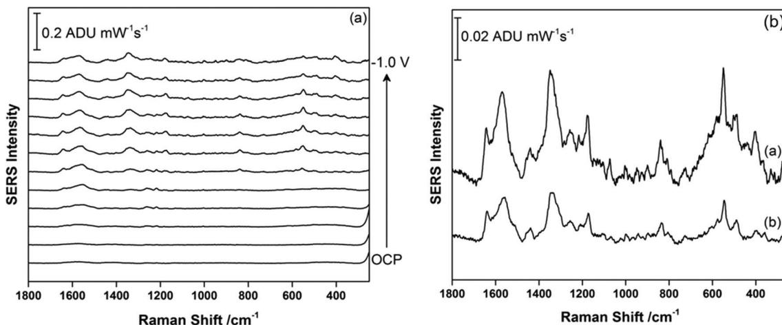
Fig. 7 (a) EC-SERS signal for THC-COOH drop-coated onto the silver electrode and measured in synthetic urine directly starting at OCP, and then stepping from 0.0 V to  $-1.0$  V in 100 mV increments. (b) Comparison of THC-COOH signal at  $-0.8$  V when the supporting electrolyte is (a) 0.1 M NaF and (b) synthetic urine. Spectra measured at 780 nm, 80 mW, 30 seconds.
