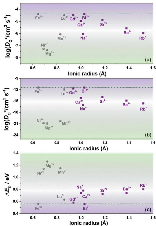
Fig. 4 Oxygen diffusion in substituted, rhombohedral BiFeO<sub>3</sub>: (a)  $D_{\text{O}}^*$  extrapolated to  $T = 1000$  K; (b)  $D_{\text{O}}^*$  extrapolated to  $T = 300$  K; (c) activation energy of diffusion. The dashed lines correspond to the values for pure BFO (Bi<sup>3+</sup> and Fe<sup>3+</sup> are also plotted for reference). Purple denotes substituents for the A site, whilst silver denotes substituents for the B site.
