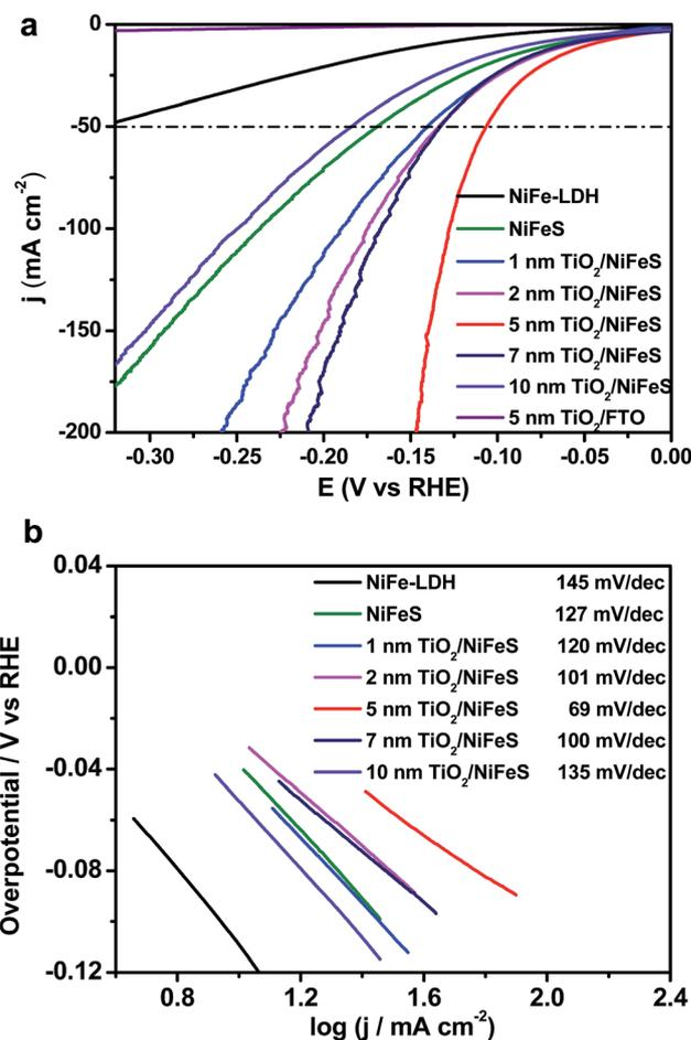
Fig. 2 Linear sweep voltammetry (LSV) curves (a) and the respective Tafel plots (b) of the ALD  $\text{TiO}_2/\text{NiFeS}$  electrodes and  $\text{TiO}_2/\text{FTO}$  (fluorine-doped tin oxide) electrodes measured in a 1 M KOH (aq) solution.
