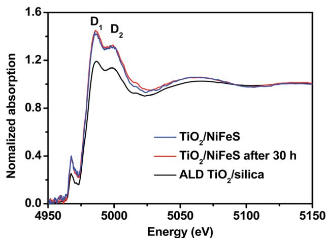
Fig. 6 Comparison of Ti K-edge X-ray absorption near edge structure (XANES) data collected on the as-prepared  $\text{TiO}_2/\text{silica}$  and 5 nm  $\text{TiO}_2/\text{NiFeS}$  nanosheets attached to Ni foam, before and after 30 hours of HER operation.
