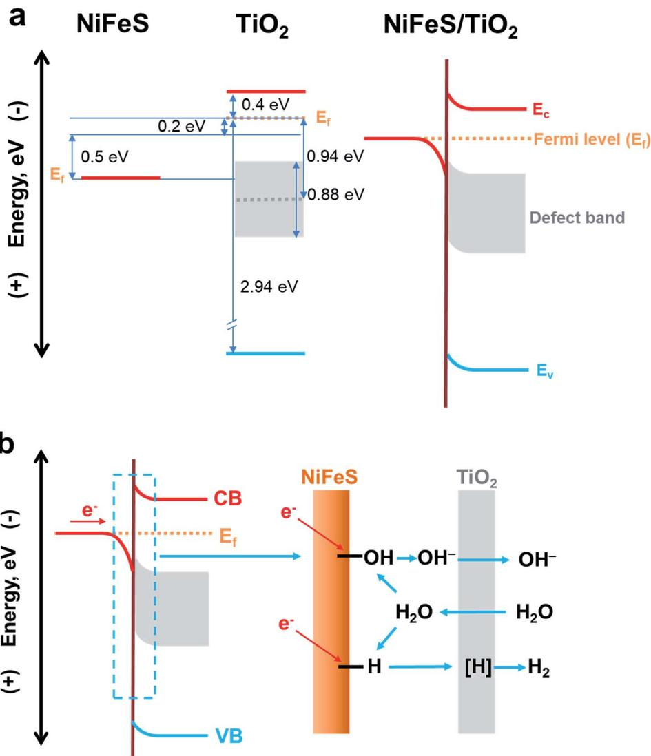
Fig. 5 (a) Energy-band diagrams of the TiO<sub>2</sub>/NiFeS interfaces. (b) Schematic illustration of the NiFeS/TiO<sub>2</sub> buried interface for boosting HER activity.
