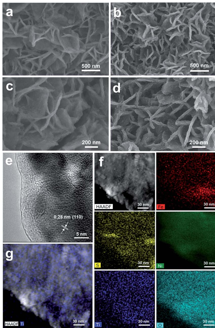
**Fig. 3** Structural and elemental characterizations of the as-synthesized NiFeS (a and c) and 5 nm ALD TiO<sub>2</sub> grown on the NiFeS nanosheets by scanning electron microscopy (SEM) (b and d), and the high-resolution transmission electron microscopy (HRTEM) image (e), high-angle annual dark-field scanning transmission electron microscopy (HAADF-STEM) image, and energy dispersive X-ray spectroscopy (EDX) elemental mapping images of the 5 nm TiO<sub>2</sub>/NiFeS structure (f and g).
