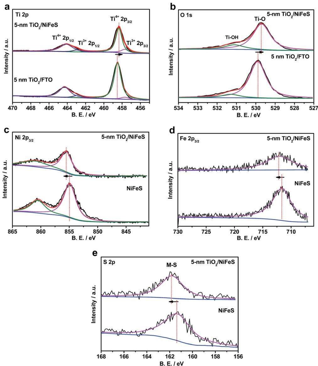
Fig. 4 X-ray photoelectron spectroscopy (XPS) spectra of Ti 2p (a) and O 1s (b) core-level photoemissions for the 5 nm ALD TiO<sub>2</sub> grown on the NiFeS and FTO substrates, and XPS spectra of Ni 2p (c), Fe 2p (d), and S 2p (e) core-level photoemissions comparing the 5 nm TiO<sub>2</sub>/NiFeS and bare NiFeS samples (blue represents the background. Black represents the raw data. The other colours represent fitting curves. The XPS measurement error for binding energies is below 0.03 eV).
