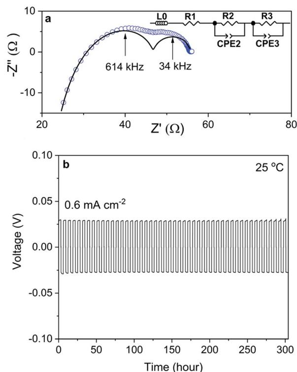
Fig. 5 (a) Experimental Nyquist plot (blue circle) of the impedance spectra recorded at  $25^{\circ}\text{C}$  with a sodium electrode normal-frequency analyzer, together with the simulated data (solid line) for NZSP0.4 (diameter of 1.03 cm and thickness of 0.185 cm). (b) Galvanostatic cycling of Na/NZSP0.4/Na at  $0.6 \text{ mA cm}^{-2}$  for 300 h at  $1.8 \text{ mA h cm}^{-2}$  per charge (discharge).
