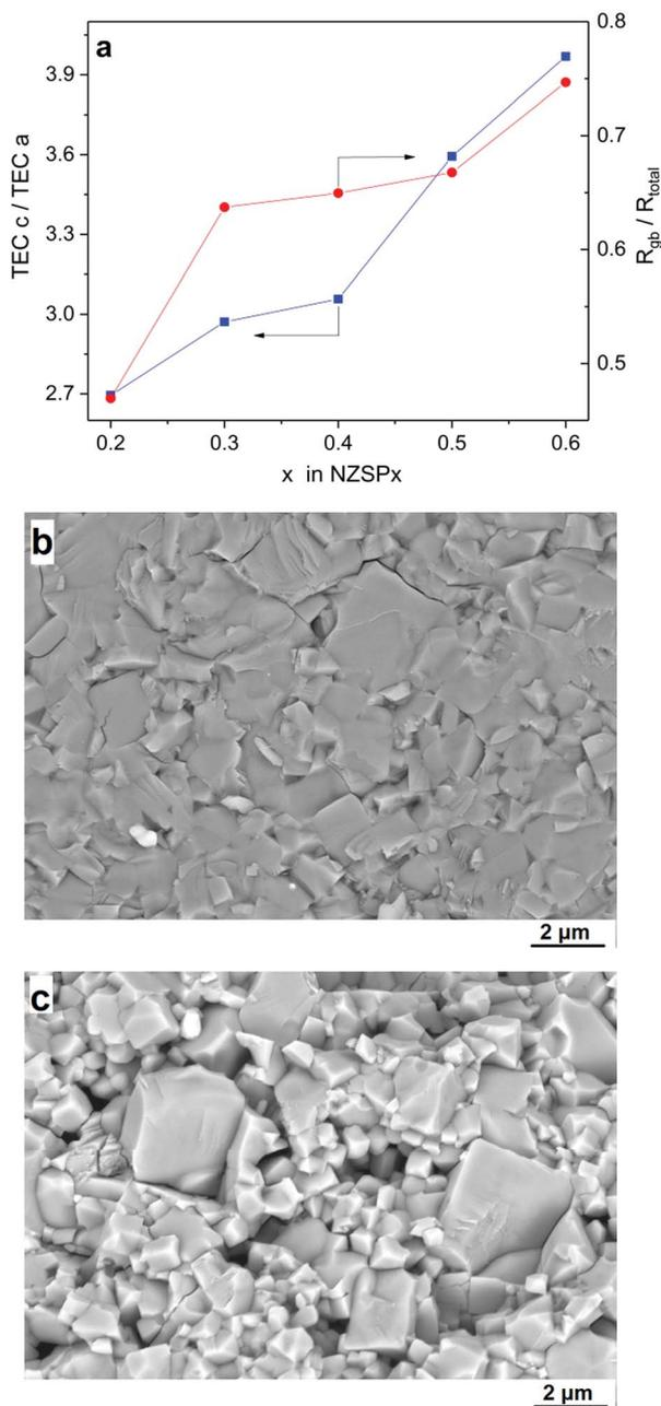
Fig. 3 (a) The comparison of TEA (expressed as TEC of lattice parameter  $c$  divided by TEC of lattice parameter  $a$ , blue squares) and contribution of  $R_{gb}$  to  $R_{total}$  (tested at 25 °C, expressed as  $R_{gb}$  divided by  $R_{total}$ , red circles) as a function of the  $x$  value in NZSP $x$ . (b) Microstructure of NZSP0.4 sintered at 1260 °C. (c) Microstructure of NZSP0.6 sintered at 1280 °C.
