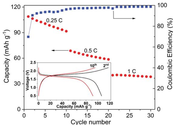
Fig. 7 Cycling performance of the full-ceramic battery operated at 28 °C. The inset displays the charge and discharge curves of the 2<sup>nd</sup> and 10<sup>th</sup> cycle at a current rate of 0.25C. The capacity in the figure indicates the specific discharge capacity of the positive electrode.
