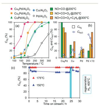
Fig. 3 (a) NO conversion to  $N_2$  during the NO reduction by CO over Pd, Cu, and Cu–Pd catalysts as a function of reaction temperature (NO, CO: 0.5%, GHSV =  $80~000~h^{-1}$ ). (b) Comparison between  $C_{N_2}$  and  $C_{N_2O}$  in NO reduction in the presence of  $O_2$  and  $C_3H_6$ . (c) Stability test for Cu<sub>5</sub>Pd/Al<sub>2</sub>O<sub>3</sub> in the NO + CO reaction at low temperatures (NO, CO: 0.5%, GHSV =  $40~000~h^{-1}$ ).
