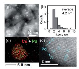
Fig. 1 (a) HAADF-STEM image of  $Cu_5Pd/Al_2O_3$  and (b) size distribution of the nanoparticles. (c) Elemental map of the Pd + Cu overlayer, as acquired by EDS. (d) High-resolution image of a single nanoparticle.
