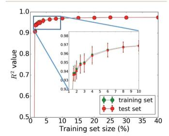
Fig. 4 Dependence of the model accuracy (measured by the correlation coefficient  $R^2$ ) on the training set size (1% corresponds to 1000 data points). The learning curve shows the mean  $R^2$  from 50 bootstrap repetitions and the standard deviation is given in the error bars. The accuracy for the training set is plotted in green, that for the test set in red.
