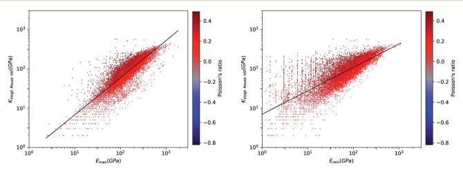
Fig. 7 Voigt-Reuss-Hill bulk modulus versus maximum (left panel) and minimum (right panel) Young's modulus for 11 764 inorganic compounds, in log-log scale. Poisson's ratio is indicated by color scale. The black line indicates the linear fit of data:  $log_{10}(K_{VRH})$  $0.95 \log_{10}(E_{\text{max}}) + 0.12 \ (R^2 = 0.64, \, \text{left}) \ \text{ and } \ \log_{10}(K_{\text{VRH}}) = 0.60 \ \log_{10}(E_{\text{min}}) \ + \ 0.84 \ (R^2 = 0.64, \, \text{right}).$
