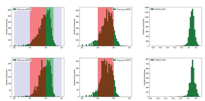
Fig. 5 Histograms of  $log(K_{VRH})$ ,  $log(G_{VRH})$ , and Poisson's ratio  $\nu$  for 8050 synthesized (top) and 3714 hypothetical (bottom) inorganic compounds.
