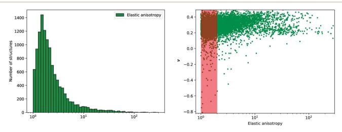
Fig. 9 Left: Histogram of elastic anisotropy  $\eta$  (in log scale) for 11 764 inorganic compounds. Right: Poisson's ratio  $\nu$  versus  $\log(\eta)$ , where the red area corresponds to anisotropy between 1 and 2.
