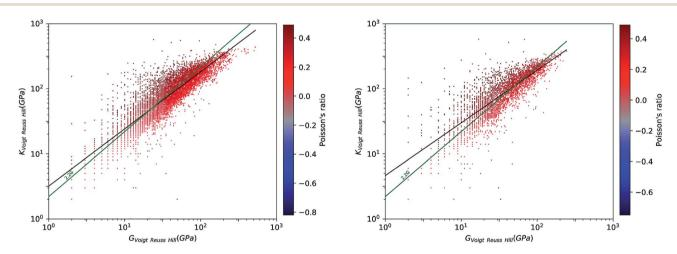
Fig. 3 Plot of bulk modulus  $K_{VRH}$  against shear modulus  $G_{VRH}$ , in log-log scale. Left: for 8050 experimentally synthesized inorganic compounds. Right: for 3714 hypothetical inorganic structures. Poisson's ratio is indicated by color scale. The black lines indicate a linear fit of data:  $log_{10}(K_{VRH}) = 0.88 log_{10}(G_{VRH}) + 0.50 (R^2 = 0.97, left)$  and  $log_{10}(K_{VRH}) = 0.81 log_{10}(G_{VRH}) + 0.67 (R^2 = 0.55, right)$ . The green lines correspond to K = 2.2G.
