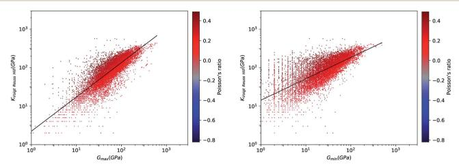
Fig. 6 Voigt-Reuss-Hill bulk modulus *versus* maximum (left panel) and minimum (right panel) shear modulus for 11 764 inorganic compounds, in log-log scale. Poisson's ratio is indicated by color scale. Black lines indicate the linear fit of data:  $\log_{10}(K_{\text{VRH}}) = 0.89 \log_{10}(G_{\text{max}}) + 0.35 (R^2 = 0.64, \text{left})$  and  $\log_{10}(K_{\text{VRH}}) = 0.56 \log_{10}(G_{\text{min}}) + 1.15 (R^2 = 0.64, \text{right})$ .
