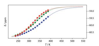
Fig. 11  $^{19}$ F NMR (500 MHz, TCE-d<sub>2</sub>, 7.4 mM) melting experiments. The lines show fitting of a two-state equilibrium isochore to the AD data (red) and a three-state isochores to the ADAD data (inner residue green, outer residue blue).
