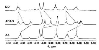
Fig. 6 Aliphatic region of the  $^{1}$ H NMR (CDCl $_{3}$ , 298 K) spectra of DD (400 MHz, 1 mM), ADAD (500 MHz, 5 mM), and AA (400 MHz, 5 mM). Chemically related signals are connected with dashed lines.
