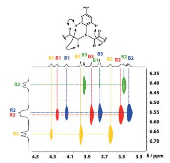
Fig. 3 Part of the  $^1\text{H}-^1\text{H}$  NOESY (500 MHz, CDCl $_3$ , 298 K, ca. 5 mM) spectrum of the ADAD 4-mer showing cross-peaks with the R2  $^1\text{H}$  signal. Signals due to different residues are distinguished by colour.
