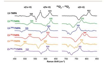
Fig. 8 Comparison of rR data ( $^{16}\text{O}_2$ – $^{18}\text{O}_2$ ) for the LS-<sup>X</sup>TMPA complexes, which are normalized to equal  $\nu$ (Fe–O) and  $\nu$ (O–O) intensities to aid in visual comparison. Isotope-sensitive features are labelled by their frequency in  $^{16}\text{O}_2$ . Note that some modes (e.g. 789 cm<sup>-1</sup> in red spectrum) are split by Fermi coupling. Asterisks (\*) denote a ferric superoxo impurity. Laser excitation was 413 nm or 780–890 nm, see ESI.†
