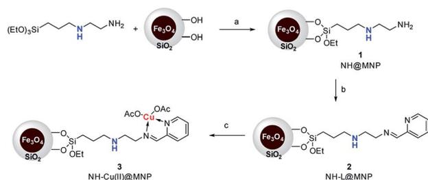
Scheme 1 Synthesis of MNP-supported bifunctional catalyst NH-Cu(II)@MNP (3). Reaction conditions: (a) toluene, N<sub>2</sub>, reflux, 24 h; (b) pyridine-2-carbaldehyde, EtOH, N<sub>2</sub>, reflux, 4 h; (c) Cu(OAc)<sub>2</sub>·H<sub>2</sub>O, acetone, N<sub>2</sub>, RT, 24 h.
