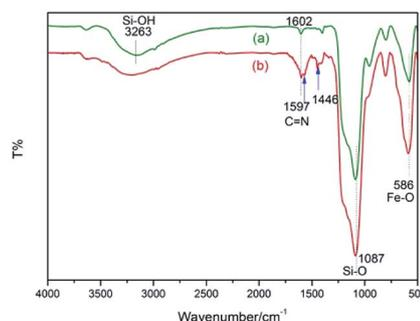
Fig. 3 FT-IR spectra of (a) Fe<sub>3</sub>O<sub>4</sub>@SiO<sub>2</sub> and (b) NH-Cu(II)@MNP.
