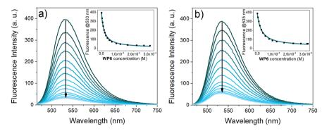
Fig. 4 Fluorescence titration of the guests (a) i2 (1  $\mu$ M,  $\lambda_{ex}$ : 433 nm) (b) i3 (1  $\mu$ M,  $\lambda_{ex}$ : 438 nm) with WP6 (0 to 300 equivalents) in 0.02 M HEPES buffer (pH 7.4). The insets show the fluorescence emission at 533 nm vs. WP6 concentration (black dots: experimental data, cyan curve: result of non-linear fitting).
