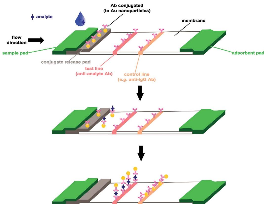
Fig. 4 An example of a lateral flow immunoassay test platform (adapted from Koczula *et al.*<sup>25</sup>). The sample solution containing the analyte is deposited on the sample pad and migrates towards the antibody biorecognition element (in this case conjugated to gold nanoparticles). The analyte-conjugated antibodies are captured at the test line (positive outcome), while antibodies which are not bound to analyte are captured at the control line (providing test validation).
