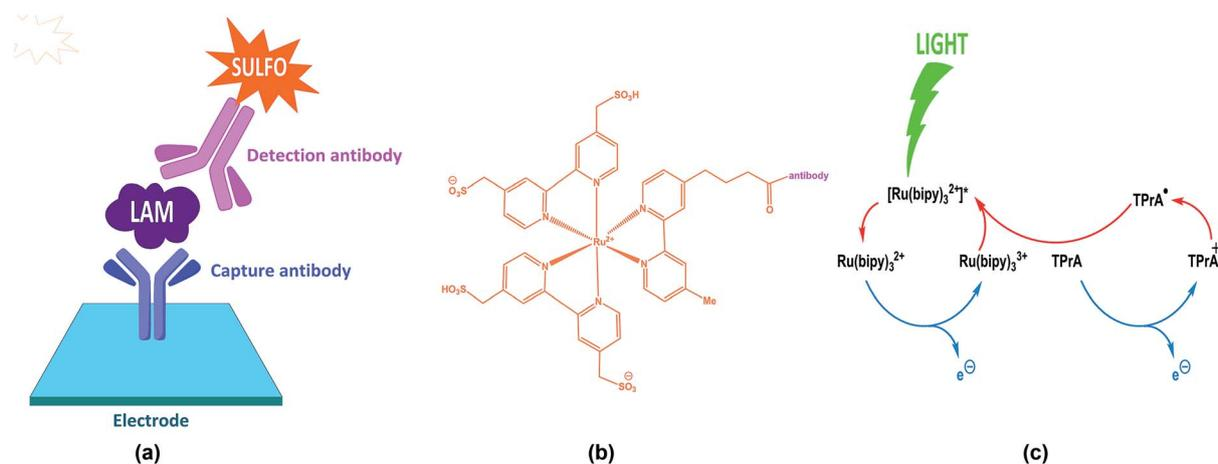
Fig. 3 Schematic of the ECL-based detection of *M. tuberculosis* through an antibody sandwich complex for the 5-methylthio-D-xylofuranose-lipoarabinomannan (MTX-LAM) epitope (adapted from [https://www.mesoscale.com/en/technical\\_resources/our\\_technology/ecl](https://www.mesoscale.com/en/technical_resources/our_technology/ecl)).<sup>24</sup>
