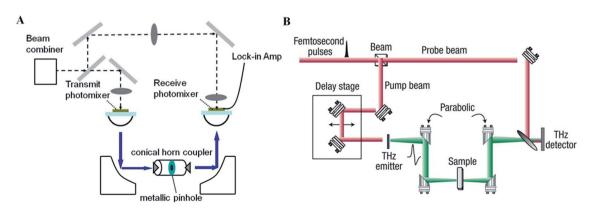
Fig. 1 Schematic illustration of THz spectroscopic instrument. (A) Photomixing spectrometer. (B) THz-TDS system.
