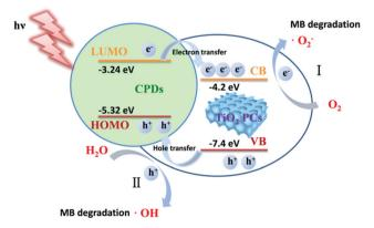
Scheme 2 Schematic photocatalytic mechanisms of CPD/TiO<sub>2</sub> PC heterostructures.
