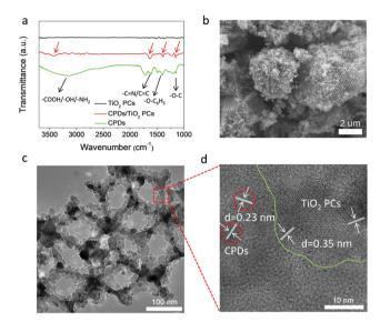
Fig. 2 Characterization of a CPD/TiO<sub>2</sub> PC heterojunction. (a) FT-IR spectra of CPDs, TiO2 PCs and CPD/TiO2 heterostructures. (b) SEM, (c) TEM and (d) HR-TEM images of CPD/TiO2 PC heterostructures.
