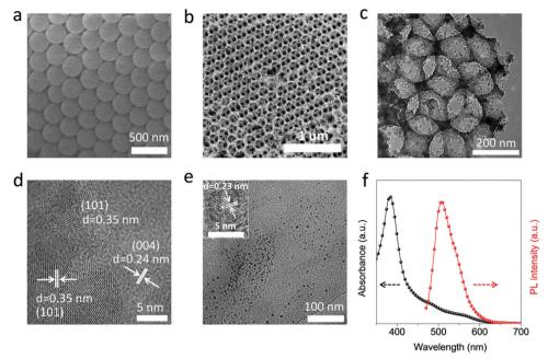
Fig. 1 Characterization of TiO<sub>2</sub> PCs and CPDs prepared from p-aminosalicylic acid and citric acid precursors. (a) SEM image of closed-packed PS microspheres. (b) SEM, (c) TEM and (d) HR-TEM images of the as-prepared TiO2 PCs. (e) TEM image of the CPDs. Inset shows the HR-TEM image of the CPDs. (f) UV-visible absorption and steady-state photoluminescence spectra of the CPDs.
