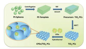
Scheme 1 Schematic procedures for the preparation of CPD/TiO<sub>2</sub> PC heterostructures. In the magnified scheme of CPD/TiO2 PC heterostructures, the size of the CPDs is enlarged to make them visible.
