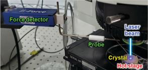
**Fig. 14** Photographs of the setup for the photoirradiation experiments. (a) Overall view and (b) expanded view around the crystal sample. A laser beam line is illustrated.
