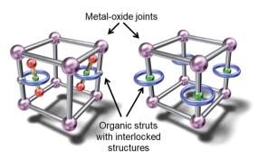
Fig. 3 Conceptual illustration of MOFs incorporating rotaxanes.
