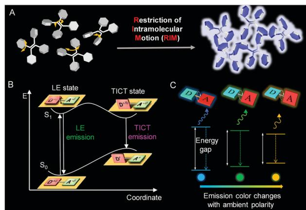
Fig. 1 A Schematic illustration showing the mechanisms of the AIE phenomenon (A). Jablonski diagrams of TICT dynamics in the donor–acceptor system (B) and (C). Reproduced from ref. 82 with permission from Wiley-VCH.
