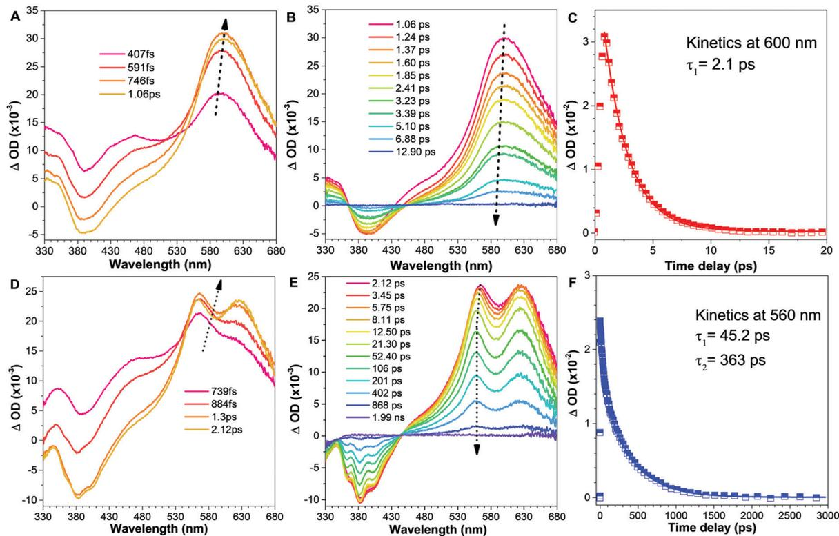
**Fig. 3** Femtosecond transient absorption (fs-TA) spectra. (A), (B) 2,4,6-TMe-DPE and (D), (E) 2,4,5-TMe-DPE in THF solution with 267 nm excitation. Kinetic traces of (C) 2,4,6-TMe-DPE at 600 nm and (F) 2,4,5-TMe-DPE at 560 nm. The solid lines indicate a fitting of the data using a single exponential function.
