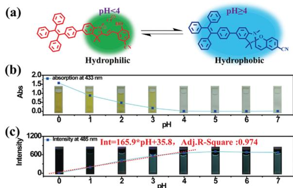
Fig. 2 (a) Illustration of switching between the ring-closed and protonated ring-open forms of **TPE-Sp-CN** at different pH values. (b) The plot of the absorption at 433 nm of the **TPE-Sp-CN** solutions (1 mL,  $1 \times 10^{-4}$  M) treated with 0.2 mL water samples with different pH values (0 to 7). (c) The plot of the emission intensity of **TPE-Sp-CN** in acid solutions ( $V_{\text{MeCN}} : V_{\text{acid water}} = 1 : 9$ ) against pH (0 to 7).
