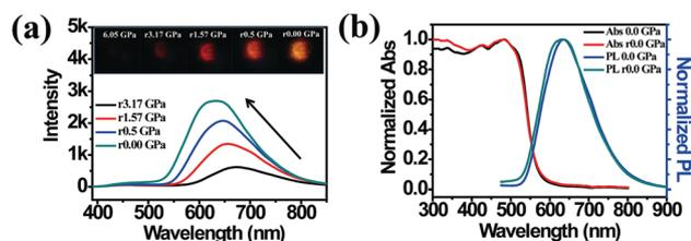
Fig. 8 (a) The *in situ* PL spectra of *c*TPE-MCH-CN during the pressure releasing process. (b) Comparison of the absorption spectra and PL spectra between the pristine state and pressure-released state.
