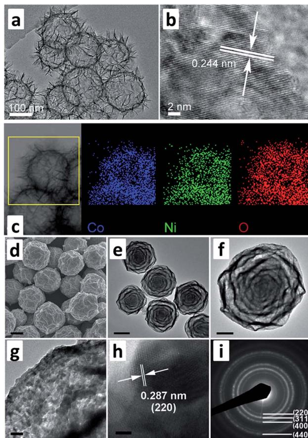
Fig. 1 (a–c) TEM images and EDS mapping of three dimensional  $\text{NiCo}_2\text{O}_4$  nanospheres, (d–i) SEM and TEM images of seven-layered Ni–Co oxide spheres derived from MOF (modified from ref. 32 and 33, copyright permission from Elsevier and Wiley-VCH, respectively).
