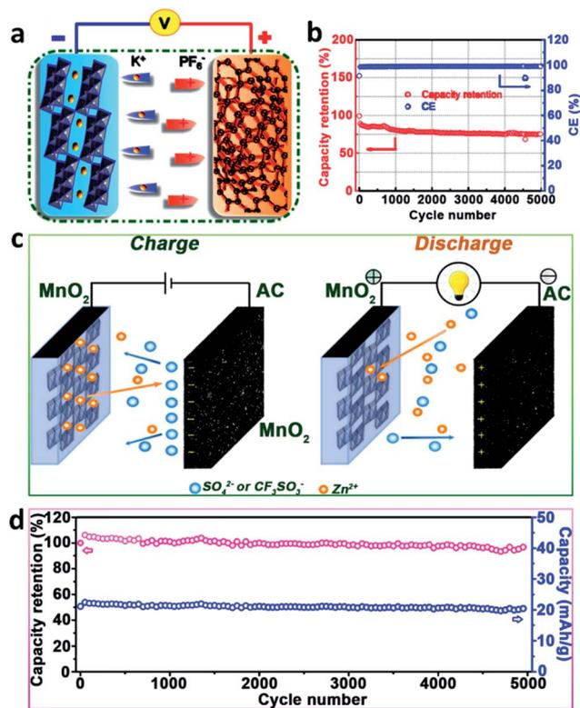
Fig. 9 (a) Schematic and (b) long-term cycling stability at the current density of  $1 \text{ A g}^{-1}$  of a NGC//KTO KIHS (modified from ref. 125, copyright permission from the American Chemical Society); (c) schematic illustration and (d) cycling stability of a designed  $\text{MnO}_2$ //AC ZIHS (modified from ref. 126, copyright permission from Elsevier).
