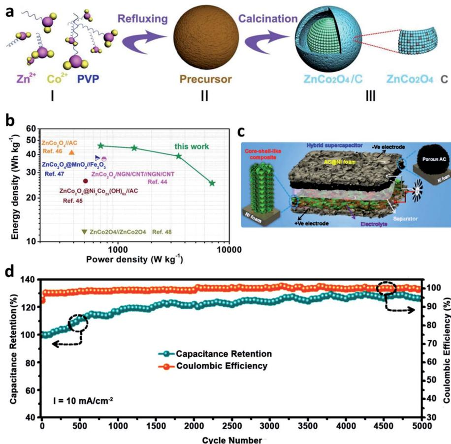
Fig. 4 (a) Scheme of the synthesis a yolk-shell structure  $\text{ZnCo}_2\text{O}_4$  material, (b) Ragone plots of AACSs (modified from ref. 85, copyright permission from the Royal Society of Chemistry); (c) illustration for the preparation process and (d) cycling stability of core-shell-like  $\text{NiO}@\text{Co}_3\text{O}_4\text{-NiO}$  FTN/Ni foam (modified from ref. 88, copyright permission from Elsevier).
