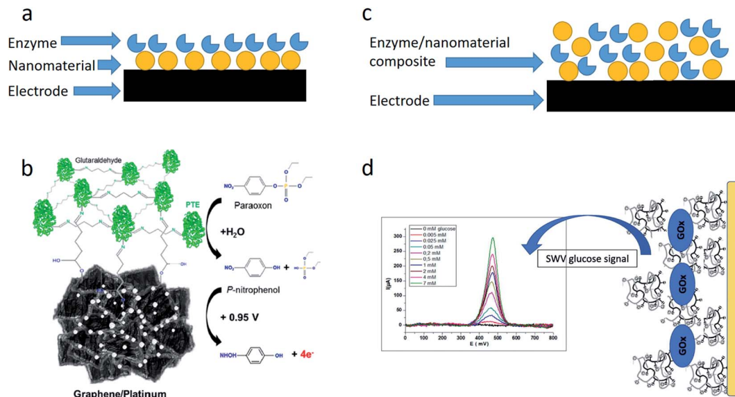
Fig. 1 Ways of embedding NMs in the enzyme-based biosensors. (a) Enzyme immobilization on the NM-modified electrode. (b) Schematic of the biosensor based on phosphotriesterase (PTE) immobilized via glutaraldehyde on the graphene surface with platinum nanoparticles. Reprinted with permission from J. A. Hondred, J. C. Breger, N. J. Alves, S. A. Trammell, S. A. Walper, I. L. Medintz and J. C. Claussen, Printed Graphene Electrochemical Biosensors Fabricated by Inkjet Maskless Lithography for Rapid and Sensitive Detection of Organophosphates , ACS Applied Materials & Interfaces , 2018, 10, 11125–11134. Copyright 2018 American Chemical Society. 25 (c) Enzyme/NM co-immobilization on the electrode. (d) Schematic of the biosensor based on glucose oxidase encapsulated in a chitosan-kappa-carrageenan bionanocomposite. Reprinted from Material Science and Engineering: C , 95, I. Rassas, M. Braiek, A. Bonhomme, F. Bessueille, G. Rafin, H. Majdoub, and N. Jaffrezic-Renault, Voltammetric glucose biosensor based on glucose oxidase encapsulation in a chitosan-kappa-carrageenan polyelectrolyte complex , 152–159, Copyright (2018), with permission from Elsevier. 26
