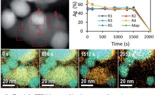
Fig. 3 Top left: STEM image of in situ energy dispersive spectroscopy showing different regions (R1 to R5) where the atomic composition spectrum was acquired. Top right: atomic composition evolution obtained by means of different regions R1 to R5 and the full map composition. Bottom: in situ energy dispersive spectroscopy showing composition variation for 2053 s. Cyan color corresponds to silver atoms and orange color corresponds to chlorine atom.
