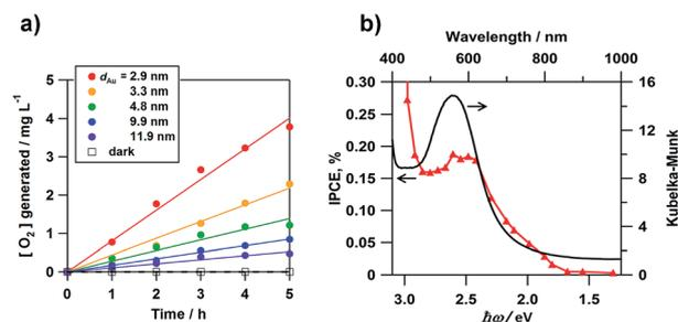
Fig. 3 (a) Time courses for the rate of  $\text{O}_2$  generation. (b) IPCE action spectrum for the photoelectrochemical WOR of the Au/ $\text{TiO}_2$ /FTO photoelectrodes with the absorption spectrum for comparison. Figure (a) is taken from ref. 41.
