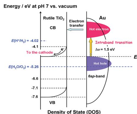
Scheme 2 Energy diagram of the Au/ $\text{TiO}_2$  plasmonic electrode with the density of states of  $\text{TiO}_2$  and energy distribution of the hot carriers in Au NPs with the intraband transition *via* the surface plasmon decay.
