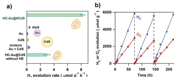
Fig. 5 (a) The comparison of the  $\text{H}_2$  evolution rate for HC-Au( $d_{\text{Au}} = 5.5$  nm)@#CdS( $\text{ICdS} = 1.9$  nm), Au colloid, CdS, and a mixture of Au and CdS under red-light illumination ( $\lambda_{\text{ex}} = 640$  nm) or dark conditions. (b) Repeated water splitting by HC-Au( $d_{\text{Au}} = 12.1$  nm)@#CdS( $\text{ICdS} = 2.1$  nm) under red-light illumination. Figures are taken from ref. 59.
