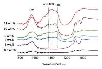
Fig. 6 FTIR spectra of the Zn-HPW/TiO<sub>2</sub> catalysts with different Zn contents. The spectra were recorded without preliminary pretreatment and are offset for clarity.
