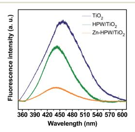
Fig. 5 Photoluminescence spectra of  ${\rm TiO_2}$ , HPW and Zn containing catalysts.
