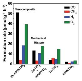
Fig. 4 CO, CH<sub>4</sub>, H<sub>2</sub> and O<sub>2</sub> formation rates over Zn–HPW/TiO<sub>2</sub>, Zn/TiO<sub>2</sub>, HPW/TiO<sub>2</sub> and a mechanical mixture of Zn/TiO<sub>2</sub> + HPW/TiO<sub>2</sub> in the photocatalytic CO<sub>2</sub> reduction. Reaction conditions: catalyst, 0.1 g; gas phase pressure, CO<sub>2</sub> 0.2 MPa; H<sub>2</sub>O, 15 mL; irradiation time, 6 h.
