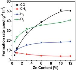
Fig. 3 CO, CH<sub>4</sub>,  $H_2$  and  $O_2$  formation rates over Zn–HPW/TiO<sub>2</sub> catalysts with different Zn loadings. Reaction conditions: catalyst, 0.1 g; gas phase pressure, CO<sub>2</sub> 0.2 MPa;  $H_2O$ , 15 mL; irradiation time, 6 h.
