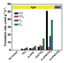
Fig. 2 CO,  $CH_4$ ,  $H_2$  and  $O_2$  formation rates over  $TiO_2$ , HPW and Zn containing catalysts in the photocatalytic reduction of  $CO_2$  in water. Reaction conditions: catalyst, 0.1 g; gas phase pressure,  $CO_2$  0.2 MPa;  $H_2O$ , 15 mL; irradiation time, 6 h.
