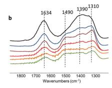
Fig. 11 In situ FTIR spectra of the  $Zn-HPW/TiO_2$  catalyst in the region of stretching vibrations of hydroxyl groups (a) and carbonates (b) measured under light at different reaction times in  $CO_2$  and  $H_2O$  vapor. The spectra are offset for clarity.
