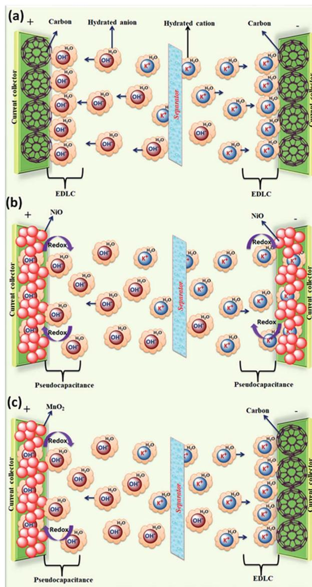
Fig. 6 Graphical representation of reaction mechanism between alkaline electrolyte (KOH) and carbon-MnO<sub>2</sub> electrodes for (a) EDLC (b) pseudocapacitor (c) hybrid supercapacitor.
