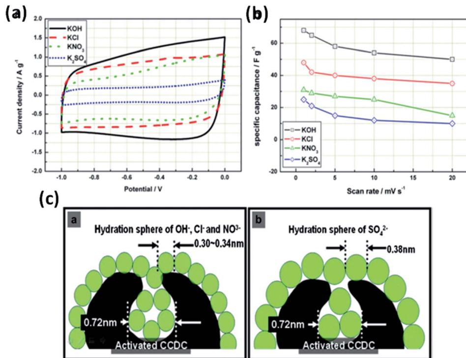
Fig. 8 (a) Cyclic voltammograms of activated CCDC supercapacitors in the aqueous electrolytes 0.5 M K<sub>2</sub>SO<sub>4</sub>, 2 M KCl, 1 M KNO<sub>3</sub> and 6 M KOH (20 mV s<sup>-1</sup>) and (b) the specific capacitance of the supercapacitor at different scan rates. (c) Schematic diagram of the relationship of hydration sphere ions and pores. This figure has been adapted from ref. 115 with permission from Elsevier.
