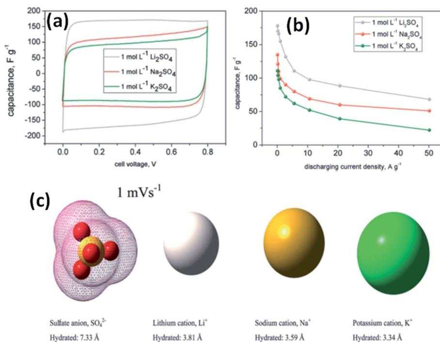
Fig. 11 (a) CV curves of a carbon based supercapacitor in 1 mol L<sup>-1</sup> alkali metal sulfate solutions (Li, Na, K) at 1 mV s<sup>-1</sup>, (b) capacitance vs. current load for different alkali metal sulfates solutions, and (c) ion shape and dimensions in aqueous solutions. This figure has been adapted from ref. 118 with permission from the Royal Society of Chemistry.
