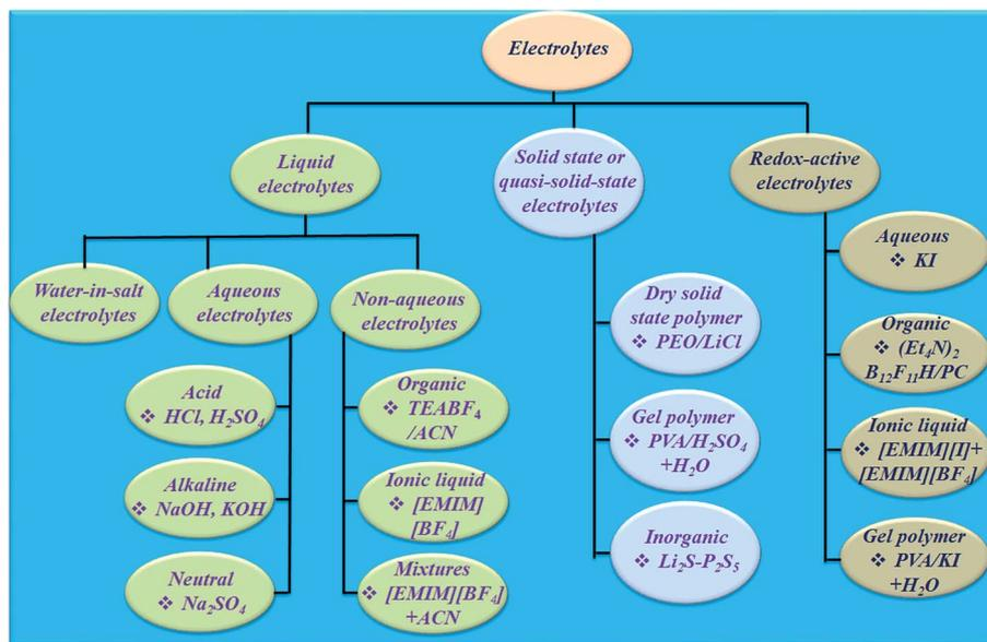
Fig. 4 Classification of electrolytes for electrochemical supercapacitors.
