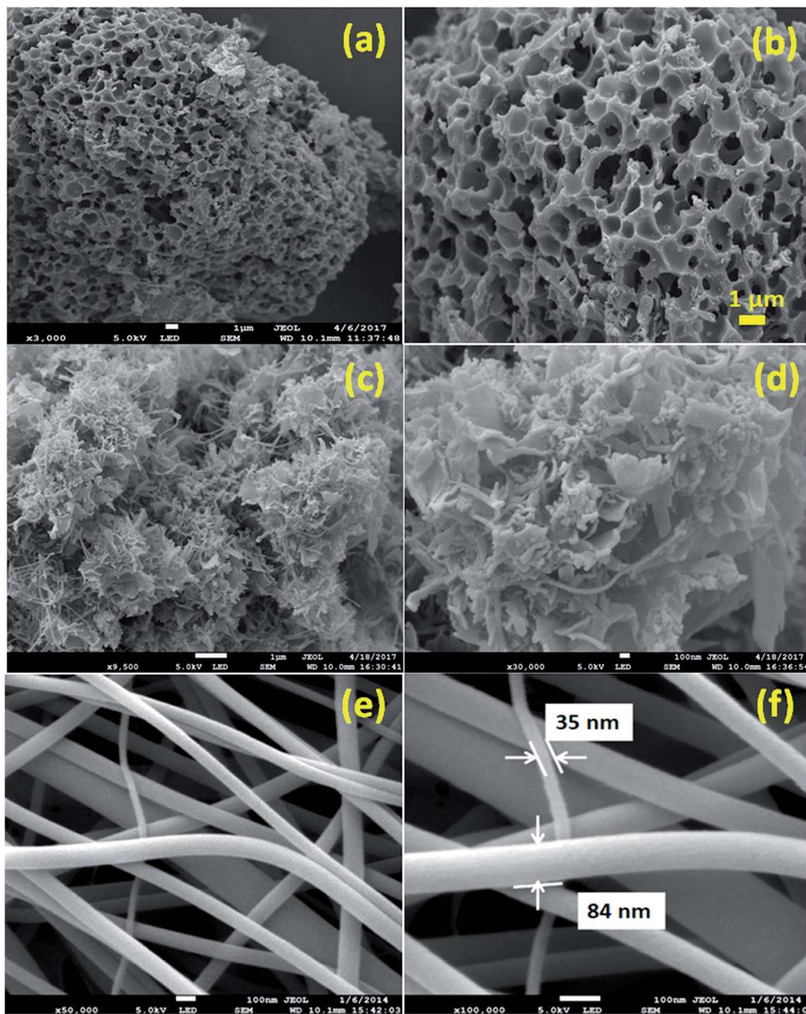
Fig. 24 FE-SEM images of various electrode materials: (a and b) porous carbon, (c and d)  $\text{SnO}_2/\text{TiO}_2$  composite flowers and (e and f)  $\text{Cu}_2\text{O}$  nanowires. (a and b) have been adapted from ref. 81 with permission from Elsevier. (c and d) have been adapted from ref. 180 and (e and f) have been adapted from ref. 29 with permission from the American Chemical Society.
