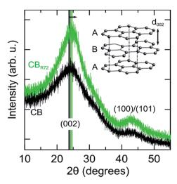
Fig. 6 XRD patterns of pristine (CB) and remotely photo-oxidized ( $CB_{R72}$ ) carbon black. The inset shows the graphene sheet-like stacking giving rise to the (002) Bragg diffraction peak, which is shifted to higher scattering angles (smaller inter-plane spacing) following photo-oxidation (arrow).
