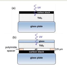
Fig. 2 Configuration of CB and TiO<sub>2</sub> layers. (a) Contact photocatalysis. (b) Remote photocatalysis experiments.
