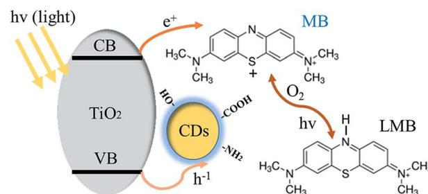
Fig. 5 Schematic of the proposed photochromic system.
