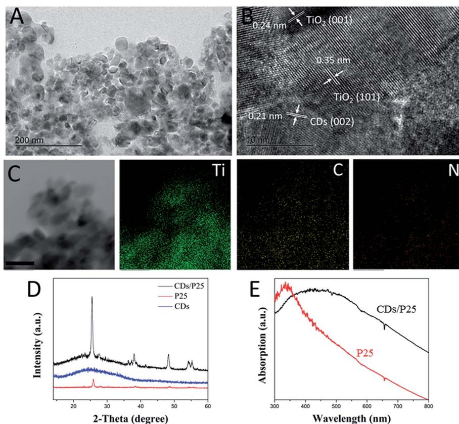
Fig. 1 (A) TEM image, (B) HRTEM image and (C) element mapping of CDs/ $\text{TiO}_2$  nanocomposites, scale bar is 50 nm. (D) XRD patterns of P25, CDs and CDs/P25. (E) UV-vis spectrum of P25 and CDs/P25.
