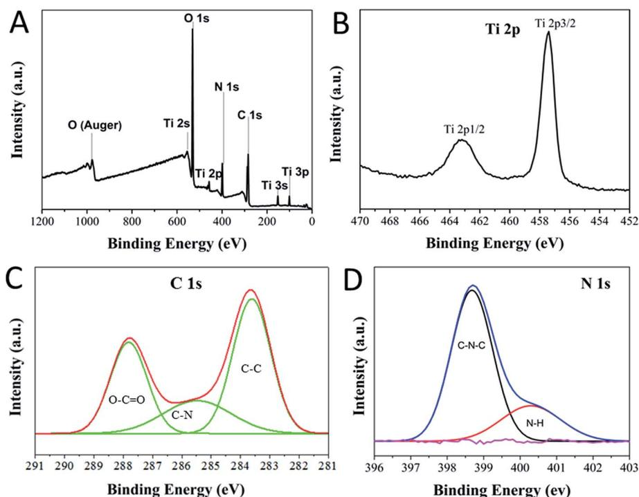
Fig. 2 XPS spectra of CDs/TiO<sub>2</sub> nanocomposites: (A) survey spectra, and (B) Ti 2p, (c) C 1s, and (d) N 1s core level spectra.
