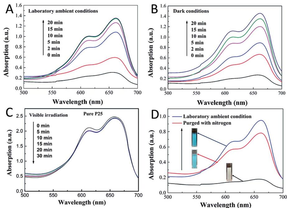
Fig. 4 (A) UV-vis spectra of the CDs/TiO<sub>2</sub> nanocomposites under recoloration process under laboratory ambient conditions and dark conditions. (B) Photocatalytic test of pure P25 nanoparticles upon UV-vis irradiation in twenty minutes. (C) UV-vis spectra of the P25 under decoloration process under visible light irradiation. (D) Recoloration process under laboratory ambient condition and purged with nitrogen.
