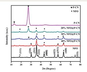
Fig. 1 XRD spectra of NFO, P-CN, and the NFO@P-CN composite.
