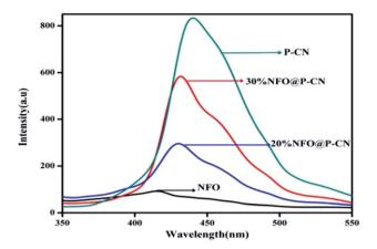
Fig. 7 PL spectra of NFO, P–CN, and 20 and 30 wt% NFO@P–CN at an excitation wavelength of  $\lambda_{\rm ex}=350$  nm.
