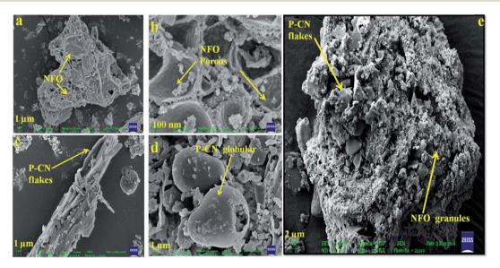
Fig. 3 (a, b) SEM image and enlarged view of NFO, (c, d) flake-like and globular structure of P-CN, and (e) 20 wt% NFO@P-CN hybrid nanomaterial.
