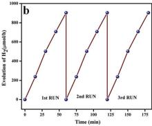
Fig. 16 (a) Rate of H<sub>2</sub> evolution shown by various prepared catalysts, (b) run graph showing the photostability towards H<sub>2</sub> evolution.
