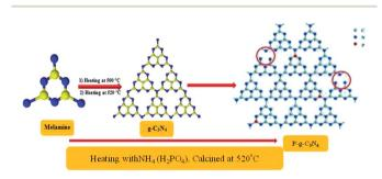
Scheme 2 Synthesis of P-g-C<sub>3</sub>N<sub>4</sub> by the calcination method.
