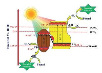
Scheme 3 Schematic presentation of the degradation of phenol and evolution of  $H_2$  over 20 wt% NFO@P-CN.
