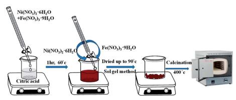
Scheme 1 Synthesis of NiFe<sub>2</sub>O<sub>4</sub> by the sol-gel method.
