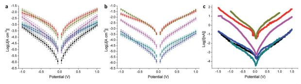
Fig. 4 Electrical characterization of tunneling junctions obtained as Au<sup>Mica</sup>/SAM//EGaln (a), Au<sup>TS</sup>/SAM//EGaln (b), and Au<sup>Mica</sup>/SAM/Au<sup>CP-AFM</sup> (c) comprising AQ (black), AC (red), APh (cyan), ABr (blue), ATTF (pink), and TCNAQ (yellow). Error bars in (a) and (b) are confidence intervals ( $\alpha = 0.05$ ). Error bars in (c) are omitted for clarity.
