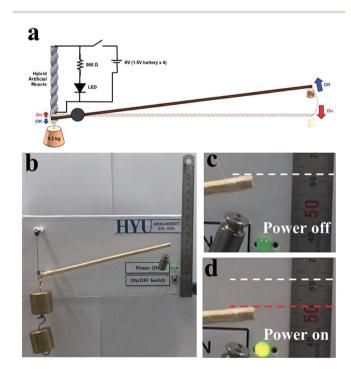
Fig. 4 Application of the HCYM actuator. A hybrid coiled yarn muscle (around 220 µm in diameter) was used to lift the pictured weight with and without an applied voltage. (a) Schematic of the circuit diagram based on electrothermal-driven contraction of the hybrid coiled yarn muscle. (b) The photograph shows the front of the HCYM. The lever arm lifted a 10 g load when the switch was turned (c) on and (d) off at 6 V using the commercial batteries (AAA type).
